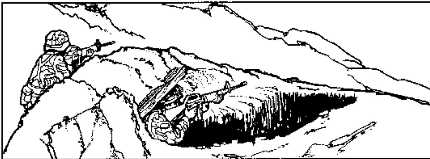
**Figure 3-2. Two-man fighting position with overhead cover.**
