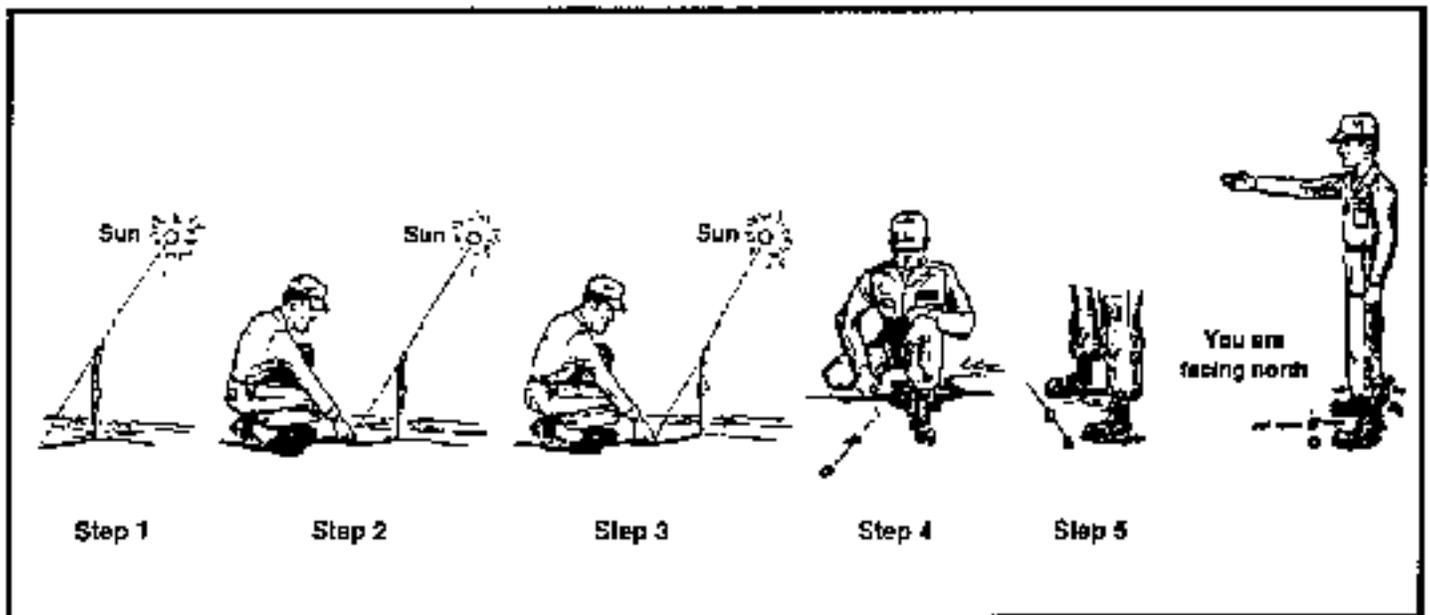
Figure 2-1. Finding direction using shadow-tip method.
