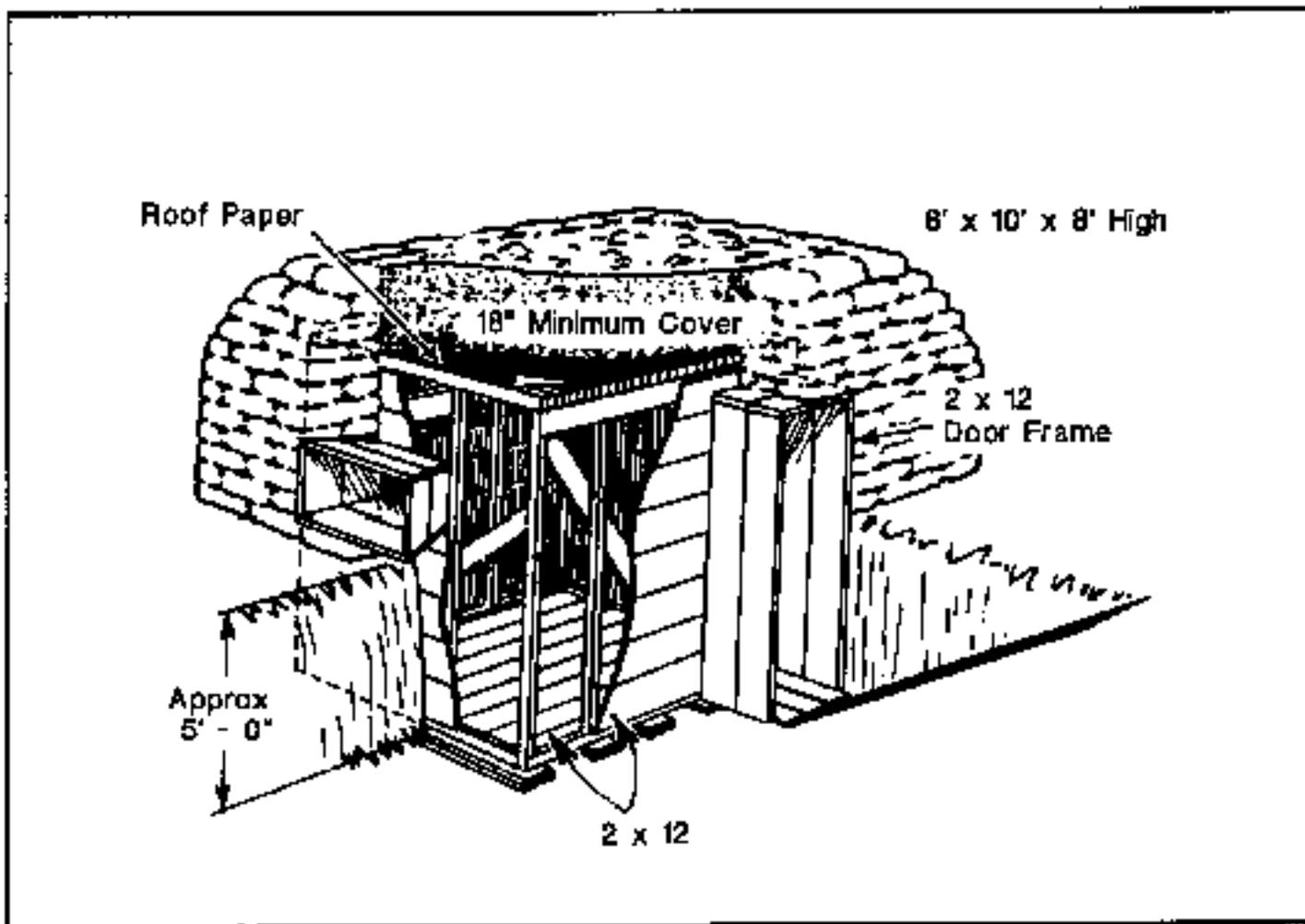
Figure 3-4. Command bunker.
