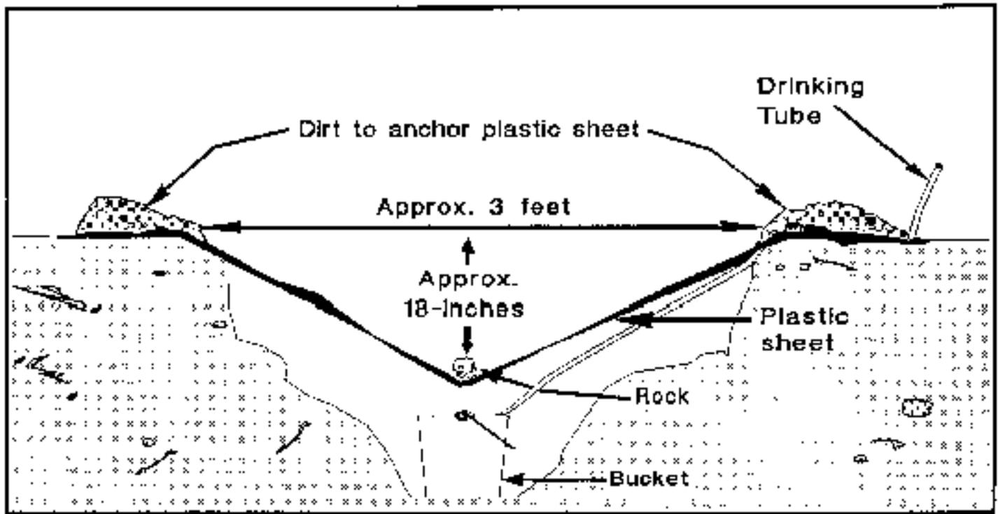
Figure 1-15. Cross-section of a survival still.
