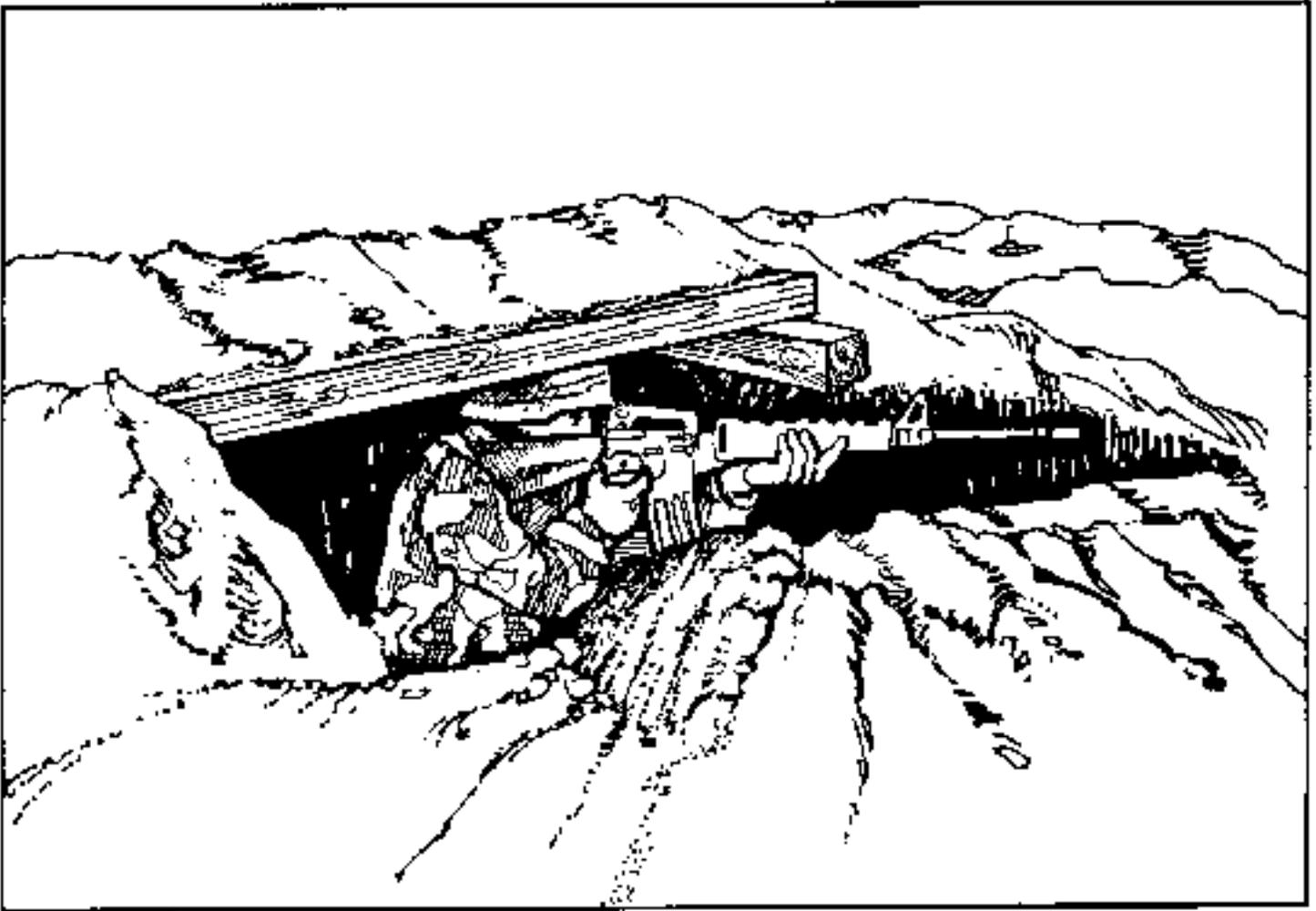
Figure 3-1. One-man fighting position with overhead cover.
